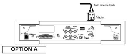
If you do not have a standard coaxial cable type of antenna or a Cable TV signal, use this option. You will need to purchase an adapter (matching transformer) like the one shown above.
